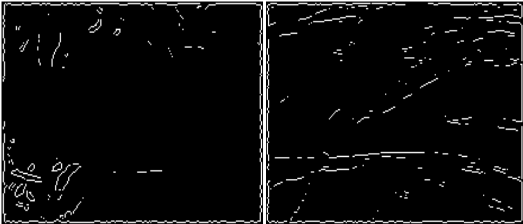
Figure 7. Black Spot after SOBEL Filter Process Figure 8. Botrytis Blight after SOBEL Filter Process
