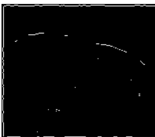
Figure 16. Rust Spores after PREWITT Filter Process
