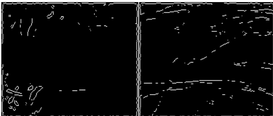
Figure 12. Black Spot after PREWITT Filter Process Figure 13. Botrytis Blight after PREWITT Filter Process
